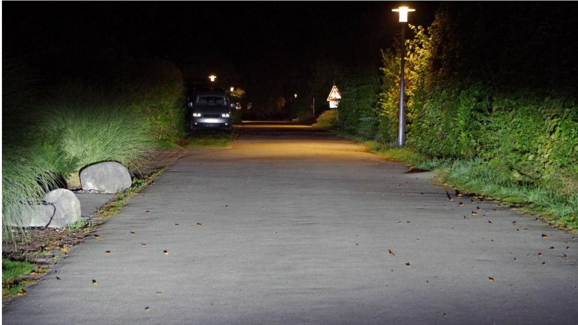
Figure 18. Street illuminated by GERG Nanolight custom road illumination module. Near area and sides are homogeneously illuminated.
