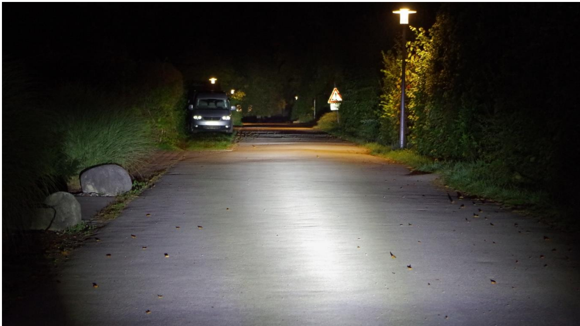
Figure 19. Street illuminated by GERG Nanolight high beam module. The area beside the cars is now fully illuminated (dark in Figure 18). Driver seat is only slightly illuminated.
